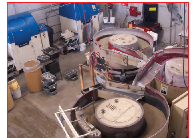
ARP's popular stainless steel engine & accessory fasteners are polished to a brilliant luster using this specialized equipment.
