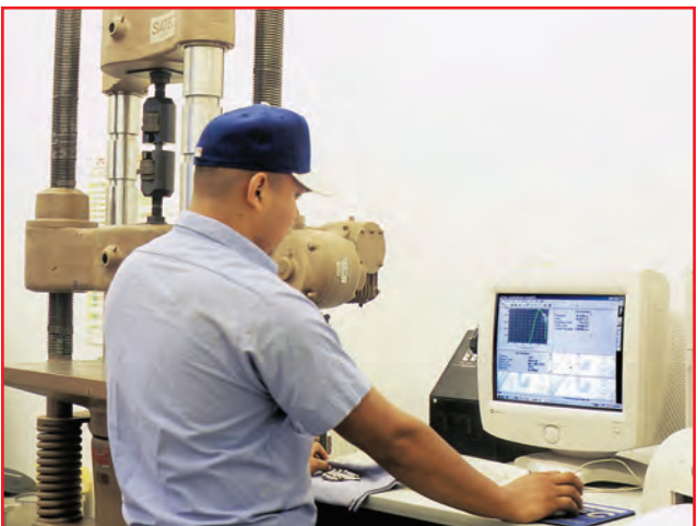
A computer-controlled Instron tensile machine is used to determine the ultimate tensile strength of studs and bolts.
