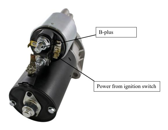
The new starter motor is threaded into the stock, which means no nuts are needed. Two M12x90 mm long bolts included.
