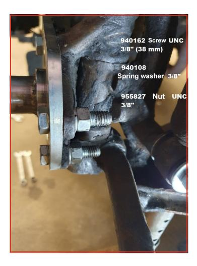
The stop screw in the spindle may need to be adjusted slightly to prevent the brake hose from touching the shock absorber.
