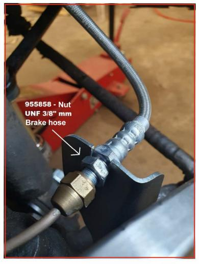
The brake hose may need to be rotated slightly to avoid contact with the tire at full steering lock.
