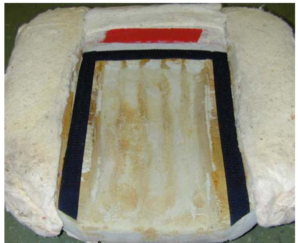
The same method used on the backrest is applied to the seat. Glue the Velcro to the frame and the upholstery.
