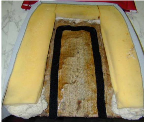
Velcro glued to the backrest frame. Match it with the backrest upholstery for correct placement..
