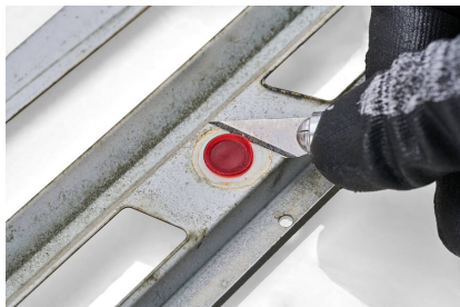
Now carefully cut off the protruding collar of the fused light windows.
